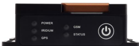
Figure 2. Status LEDs on the 9602-GSM front face.
