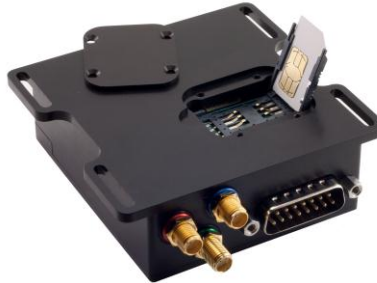
Figure 4. Location of the GSM SIM door on the 9602-GSM.
